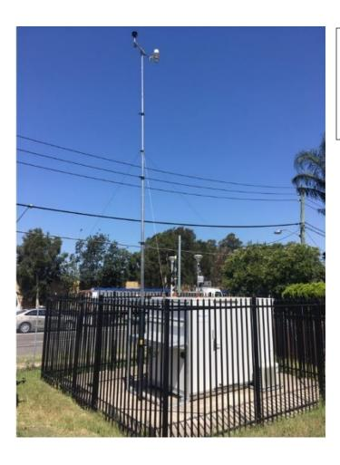
Image: An example of an air quality monitoring station. A similar unit will be installed in the Bridgewater area to monitor air quality before, during and after construction.
