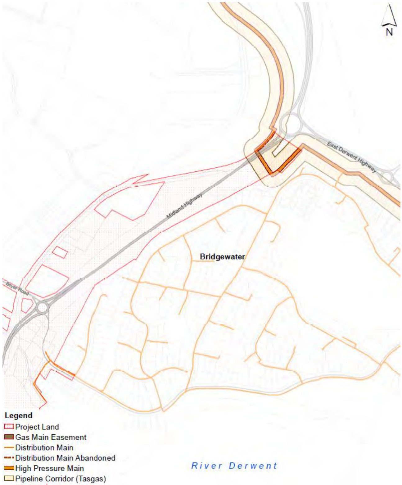
Figure 10 - Gas distribution pipe and Declared Gas Pipeline Planning Corridor
